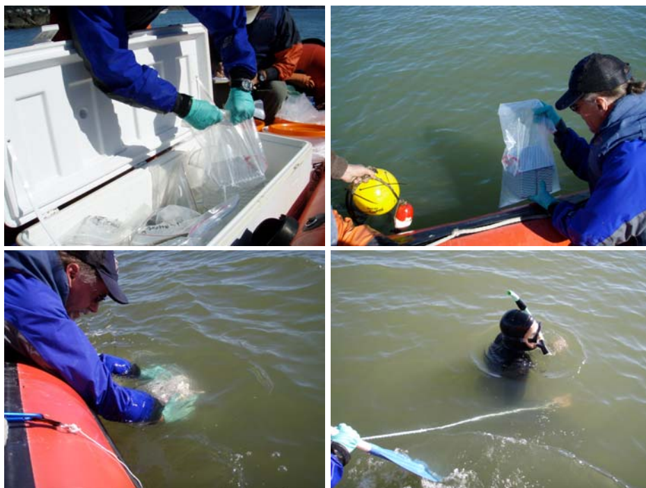
Figure 2-4: Deployment of cages: Cages were transported to the field in large ziplock bags with half-strength seawater on ice, lowered into the water in a closed bag, removed from the bag underwater and handed to a free diver to be clipped onto the mooring. Retrieval was a reverse of this process.
