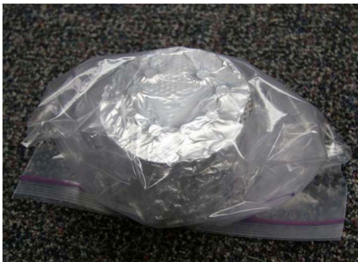
Fig. 1. Example PEMD wrapped in foil and placed in ziplock bags. This example was wrapped with a single layer of foil which has torn, illustrating the need to be careful and double wrap each canister.
